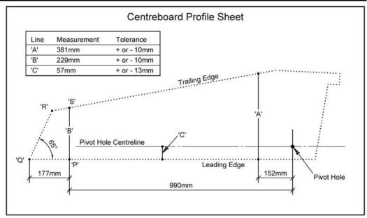
Measurements A, B and C are taken at  $90^{\circ}$  to the leading edge at the stated distance from the centre of the pivot hole. They shall be within the limits of measurement given on the Centreboard Profile Sheet.
