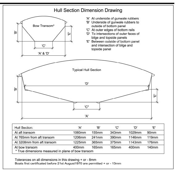
When a straight edge is placed upon either topsides, side decks, bilge panels or centre bottom panel in the same plane as the sections, no part of the surface shall be further away from the straight edge than 3mm.
